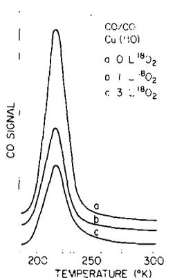
FIG. 15. The influence of surface oxygen upon the adsorption of carbon monoxide. The Cu(110) surface was oxidized at  $295 \pm 10^\circ\text{K}$  and CO was adsorbed at  $180^\circ\text{K}$ .
