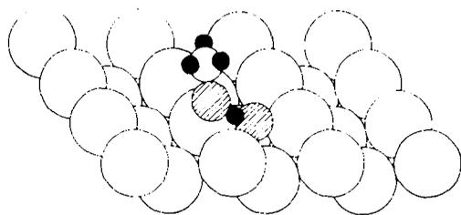
FIG. 10. A schematic representation for the adsorption of CH<sub>3</sub>OH on a partially oxidized copper(110) surface. The oxygen covalent radius was used to represent the diameter of the adsorbed oxygen atom. Small filled circle = hydrogen atom; small empty circle = carbon atom; hatched circle = oxygen atom; large empty circle = copper atom.
