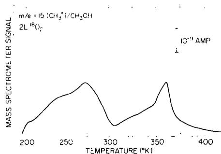
FIG. 17. The *m/e* = 15 (CH<sub>3</sub><sup>+</sup>) signal following adsorption of CH<sub>3</sub>OH at 180°K on a Cu(110) surface that was preoxidized at 295 ± 10°K with 2 Langmuirs of <sup>18</sup>O<sub>2</sub>.
