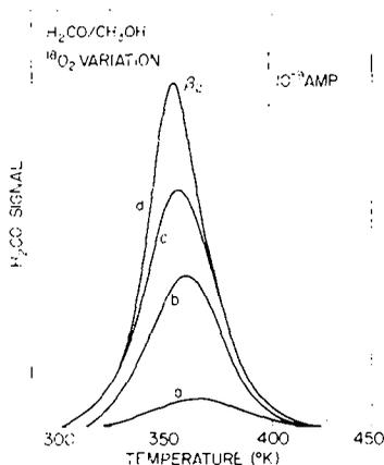
FIG. 13. The influence of low exposures of oxygen upon the H<sub>2</sub>CO flash decomposition spectrum. The Cu(110) surface was oxidized at  $295 \pm 10^\circ\text{K}$  and was given a 100-s dose of CH<sub>3</sub>OH at  $180^\circ\text{K}$ . The oxygen exposures were (a) 0, (b) 0.25, (c) 0.5, and (d) 1.0 Langmuir.
