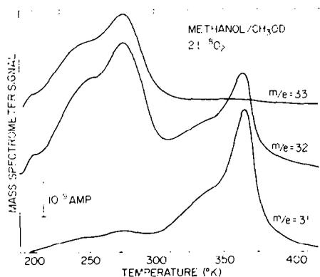
FIG. 16. The *m/e* = 33, 32, and 31 signals subsequent to the adsorption of CH<sub>3</sub>OD at 180°K on a Cu(110) surface that was predosed with 2 Langmuirs of <sup>18</sup>O<sub>2</sub> at 295 ± 10°K.
