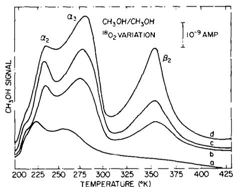
FIG. 11. The influence of low exposures of oxygen upon the  $\text{CH}_3\text{OH}$  desorption spectrum. The  $\text{Cu}(110)$  surface was oxidized at  $295 \pm 10^\circ\text{K}$  and was given a 100-s dose of  $\text{CH}_3\text{OH}$  at  $180^\circ\text{K}$ . The oxygen exposures were (a) 0, (b) 0.3, (c) 0.5, and (d) 1 Langmuir.
