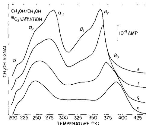
FIG. 12. The influence of high exposures of oxygen upon the CH<sub>3</sub>OH desorption spectrum. The Cu(110) surface was oxidized at  $295 \pm 10^\circ\text{K}$  and was given a 100-s dose of CH<sub>3</sub>OH at  $180^\circ\text{K}$ . The oxygen exposures were (e) 2, (f) 3, (g) 5, and (h) 10 Langmuirs.
